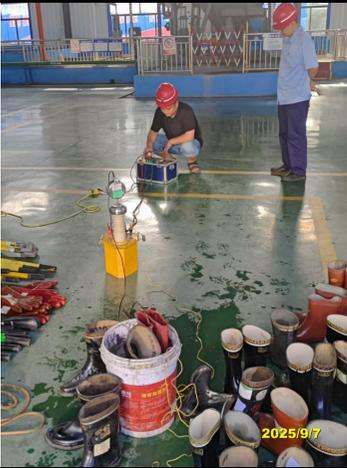
Two workers in red hard hats are in a large industrial space. One worker is kneeling and inspecting a large number of electrical insulating gloves (rubber boots) that are laid out on the floor. There are several buckets and containers around the gloves. The date '2025/9/7' is visible in the bottom right corner of the photo. |
